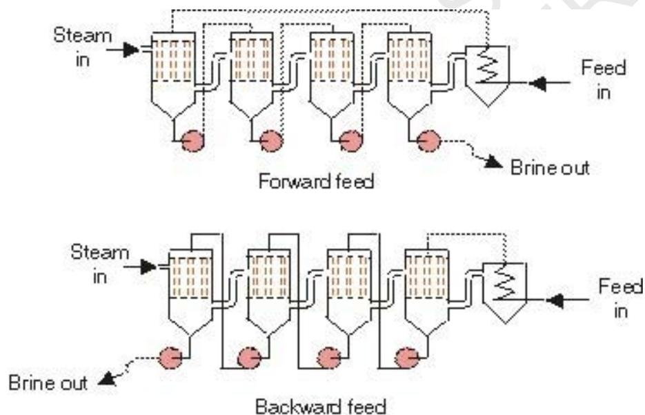
Figure 1. Types of feed for vertical tube evaporators.
