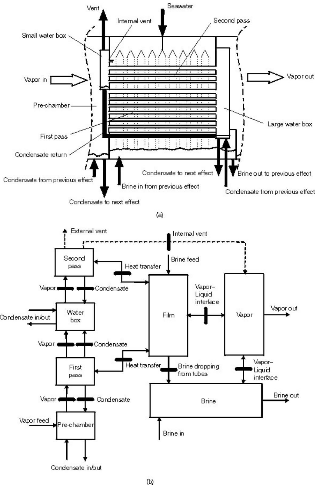
Figure 3. (a) Effect design and (b) model structure.
