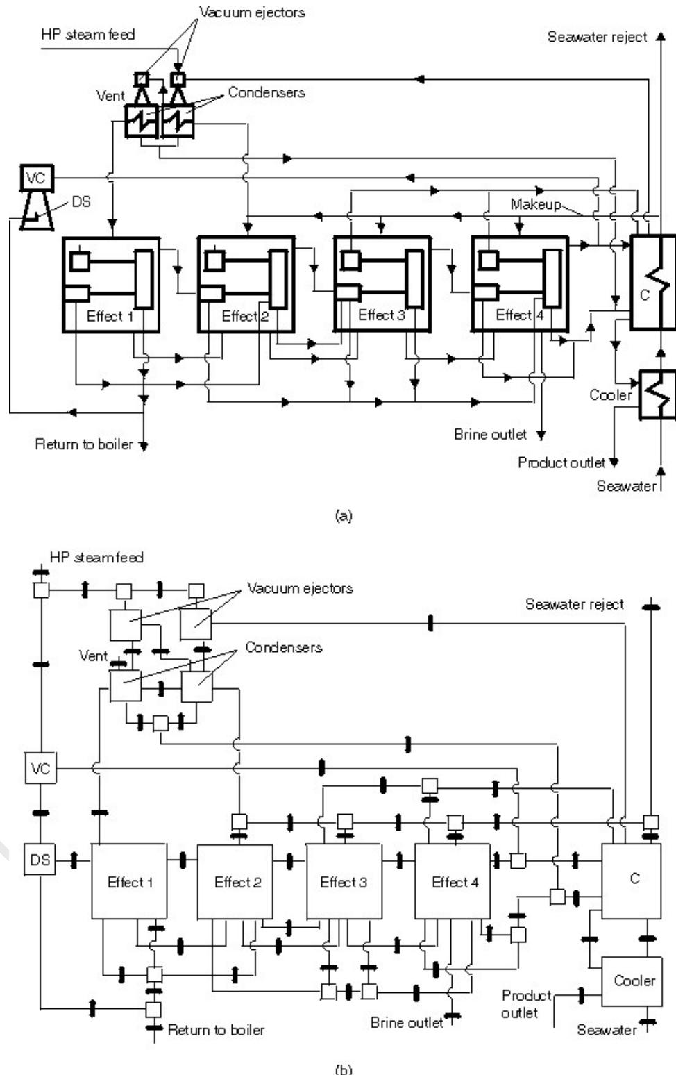
Figure 1. (a) Plant lay-out and (b) model structure. C, main condenser; VC, vapor compressor; DS, desuperheater.
