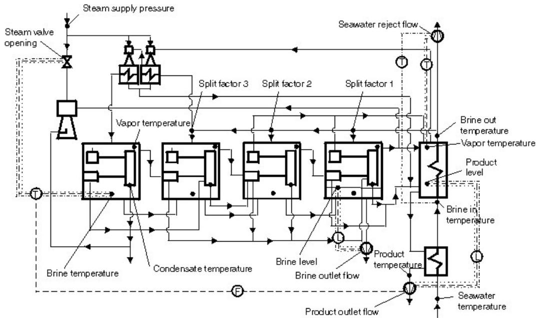
Figure 2. Control structures and measured, manipulated, and disturbance variables.
