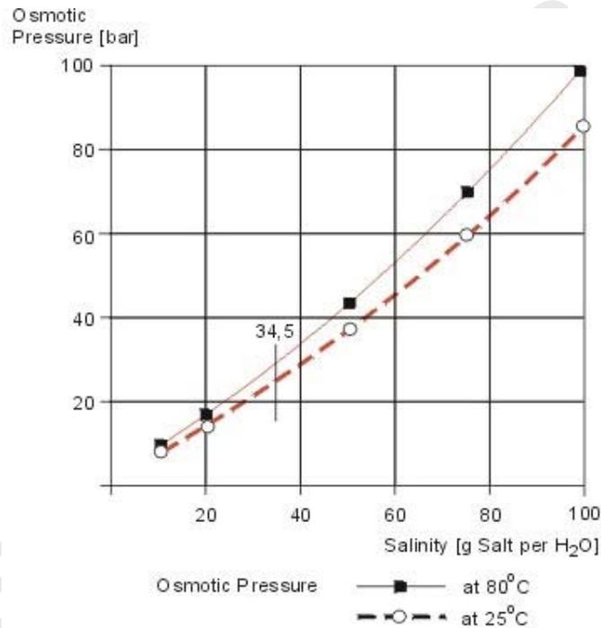
Figure 1. Osmotic pressure as a function of salinity and temperature.
