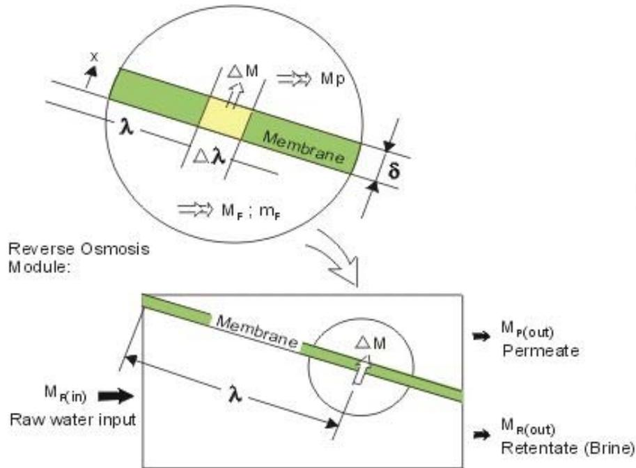
Figure 2. RO functional schematic.
