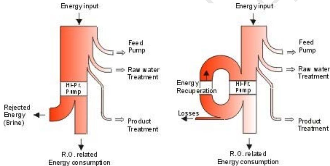
Figure 3. Energy flow diagrams: Effects of internal energy recuperation.
