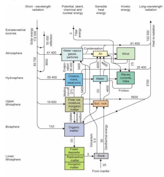
Figure 1. Energy cycle in the Earth-atmosphere system without anthropogenic interference (unit TW) (Sørensen 1979).
