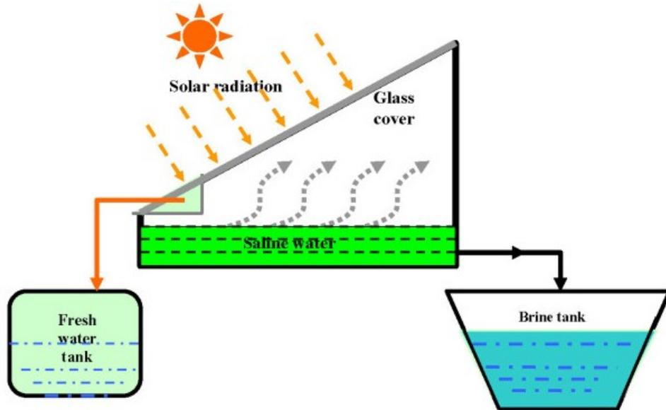
Figure 1. The schematic of a simple solar still
