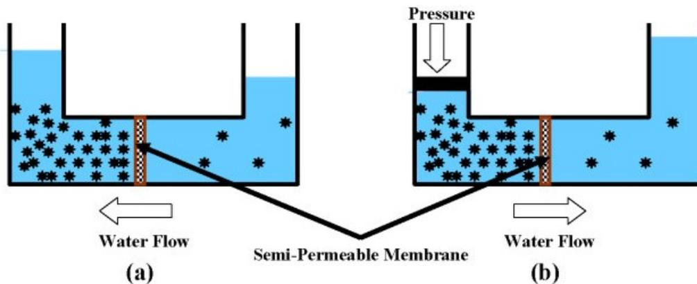
Figure 5. (a) Working principle of osmosis; (b) Working principle of reverse osmosis
