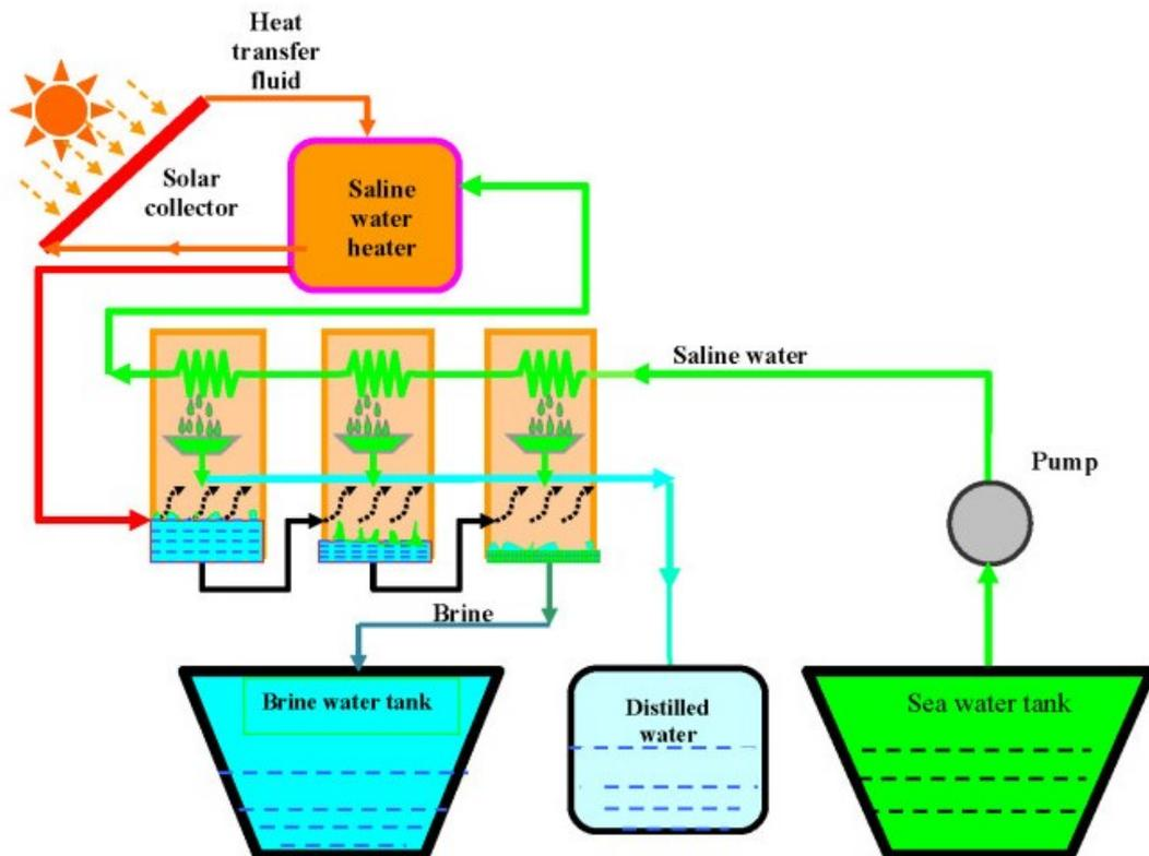
Figure 3. Solar powered multi-stage flash system
