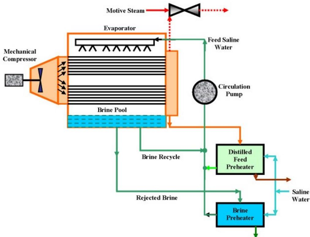
Figure 4. Vapor compression desalination system
