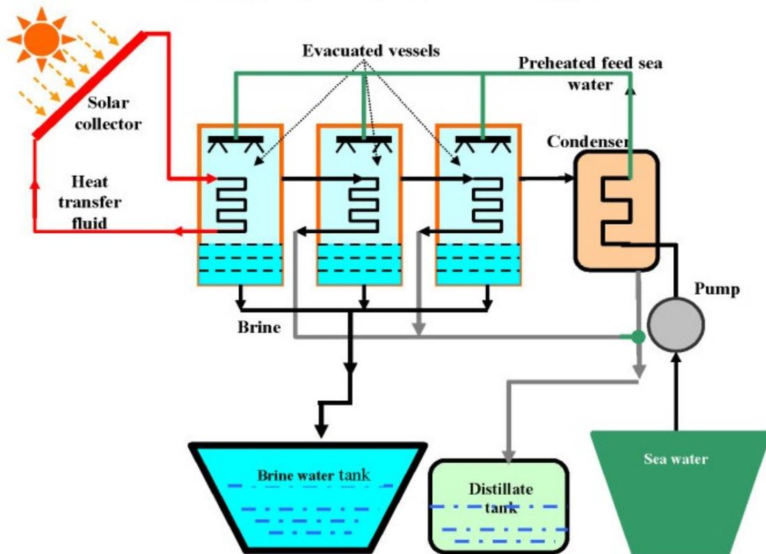
Figure 2. Solar powered multi-effect distillation unit
