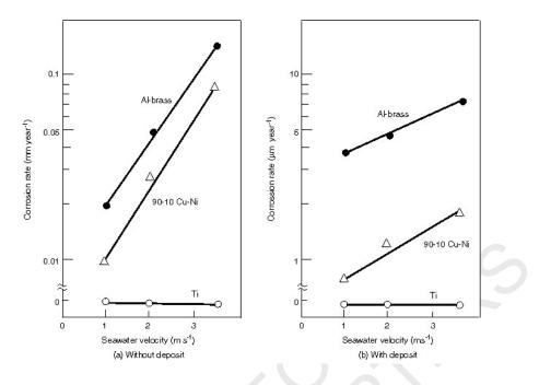
Figure 1. Corrosion rate of copper alloys and titanium with or without deposit in seawater (298 K).
