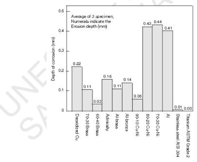
Figure 2. Resistance of various metals and alloys against vibration-type deposit attack.
