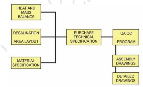
Figure 2. Schematic engineering activities sequence for auxiliary equipment procurrement.
