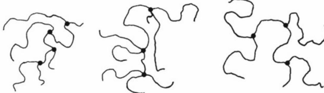
Figure 9. Sketches of branched macromolecules. a) Trifunctional branch points; b) tetrafunctional branch points; c) graft macromolecule
