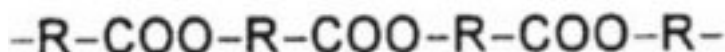
Figure 6. Formula of a section of a polyester molecule formed by polycondensation of a hydroxy acid.
