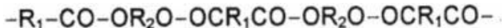
Figure 7. Formula of a section of a polyester molecule formed by polycondensation of a dicarboxylic acid and a dialcohol
